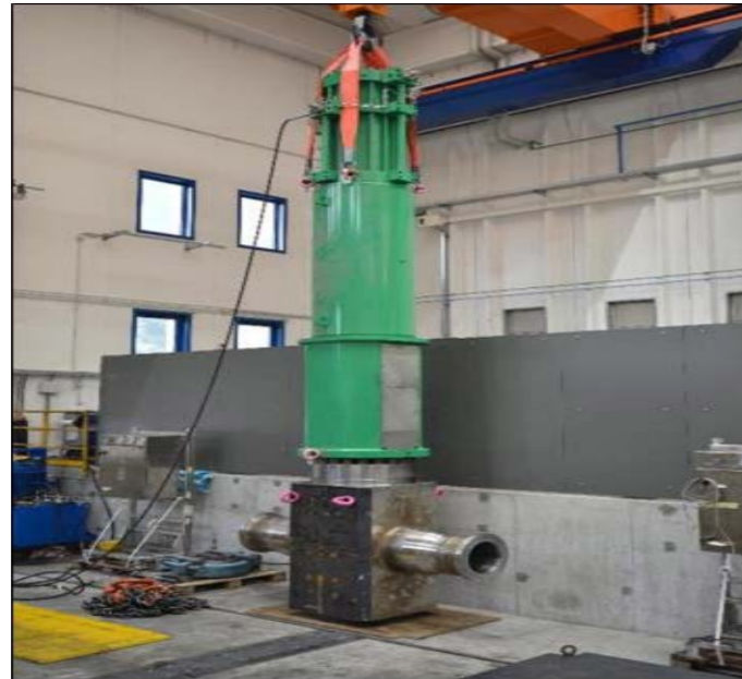
18" Class API 10000 Inconel 625 Fully cladded (33% H2S) Time to close: less than 2 seconds
