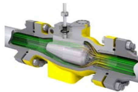
Streamlined flow path through full-port expanded body
