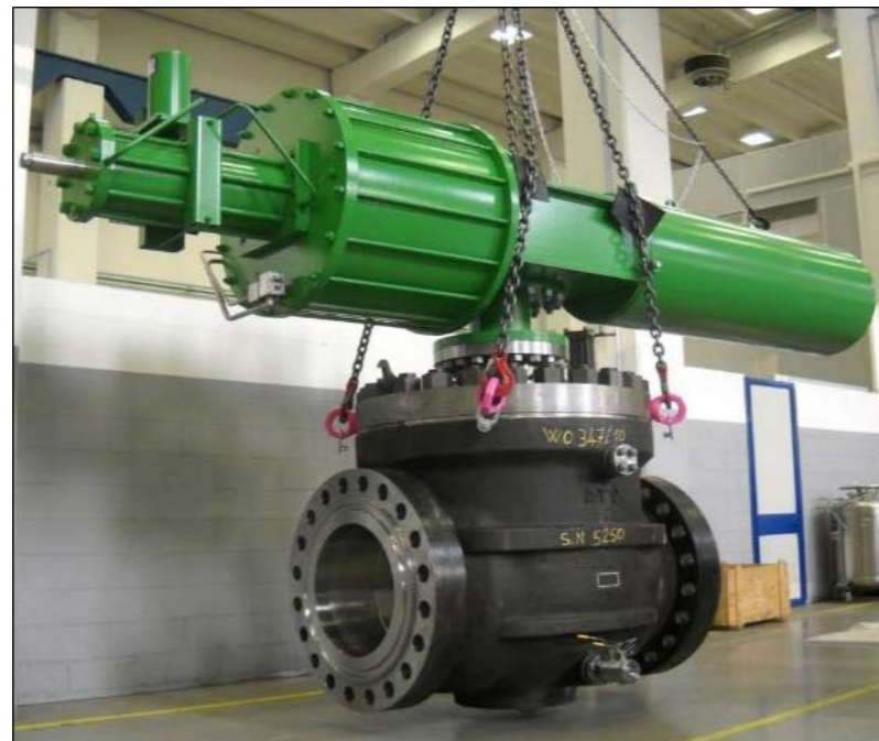
28" and 20" Class API 900 Metal Seated, Inconel 625 Fully cladded (>25% H2S)
